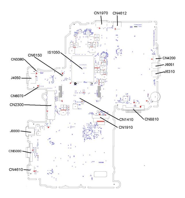
Figure B-2 System board(FW3SY\*) layout (back)
